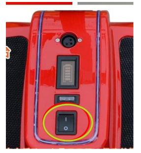
1. First Step: Turn on the power switch which between the footboards highlight in yellow circle
